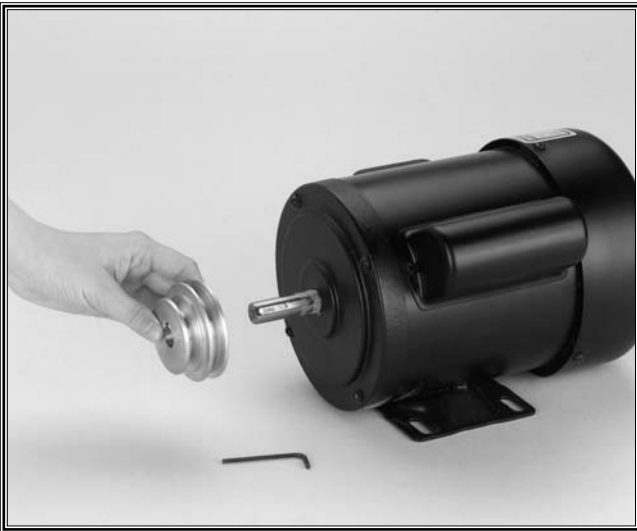
Figure 14. Installing pulley on motor.
